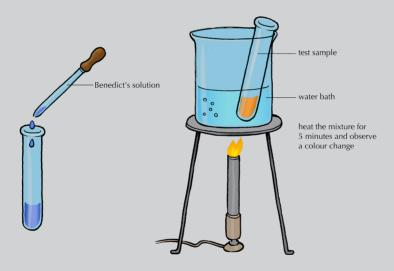
Figure 2.10: Test for reducing sugars using Benedict's test
