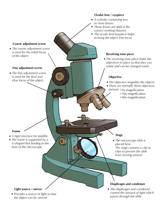
Figure 3.5: Light microscope
