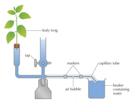
Figure 6.19: Potometer measures the rate of transpiration.
